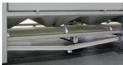
Detail of the washing system drainage.
