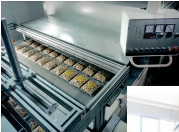
“ARF 60 kW” pasteuriser for fresh filled egg-pasta and “gnocchi” in commercial packaging (flow-pack film).
