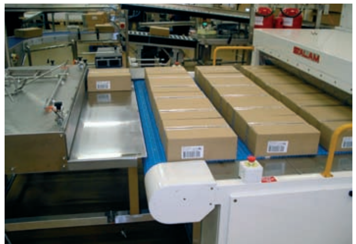
RF pasteurisation of flow-packed bread loaves (sliced toast bread) inside cardboard boxes for retail distribution.
