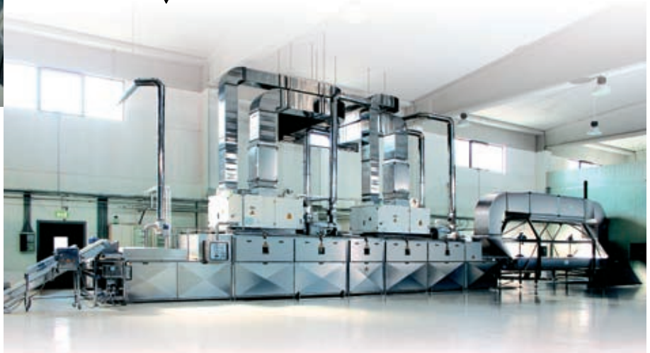
“ARF 2x40 kW” pasteurising equipment with cooler for fresh semolina pasta.
